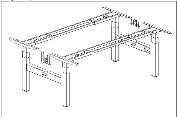
Step 7 Fix the table top with 21 pcs screws ST4x20 ,Fix the handset with 2 pcs screws with ST4x20 Install the centre bracket with 2 pcs screws M6x10  $\,$
