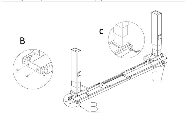
**Step 3**Install the side brackets with Screws 8 pcs M6x16,
