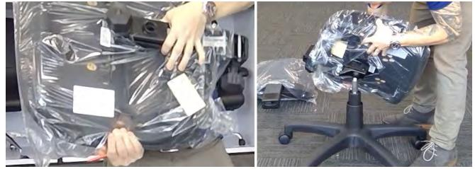
4. Slide the bar of the back into the insert of the mechanism at the back of the seat. \*But first pull out the plastic lug then slide the bar in
