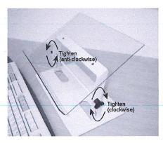
3) Use both hands to locate the correct height and angle for the Ezee Copy and then tighten the handwheels to lock the pallet in place.
