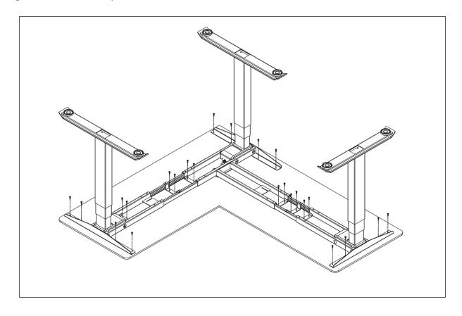
**Step 7**Mount the control box to the frame, fix the handset with 2pcs screws ST4x20.
